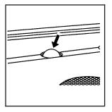
There is a light sensor located on top of the instrument panel. Make sure it is not covered, or the headlamps will come on when they are not needed.
